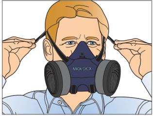
Tighten top straps first then the lower neck straps until you have a very snug and leak-free fit. Facepiece should not be loose or slide up or down the nose. Tighten by pulling on ends or loosen by pushing out on buckle tab. Do not overtighten. Further tighten top straps if necessary.
