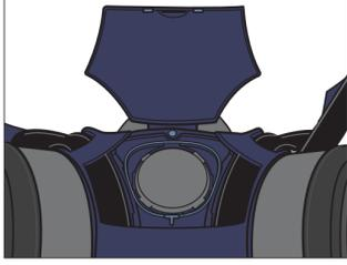
Open valve cover by pulling up on the latch. Pull the straps out from underneath the tabs of the strap channel. Close and snap shut the valve cover.
