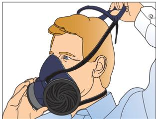
Adjust head cradle then pull the cradle to the top of the head so it rests on the crown.
