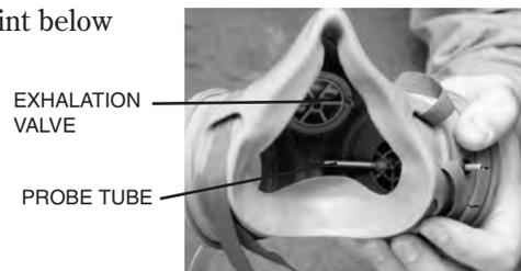
Check to see that the probed cartridge is seated properly, both inside and outside, and that it's flush against the facepiece.
