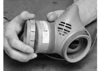
Place a new 8940 P100 Filter disk inside the retainer ring so that the side indicated is away from face. Replace the retainer ring.
