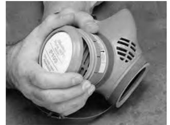
Make a careful inspection of retainer ring seal to piggyback adapter to ensure it is fully sealed.
