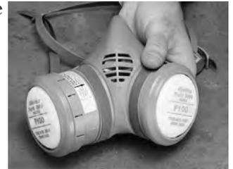
Insert 8940 P100 Filter disk into retainer ring so that the side indicated is away from face. Check to see that disks are properly sealed.
