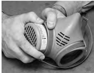
The inside probe tube must point below exhalation valve, see picture.
